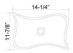
Dimensions of fixture are nominal and may vary within the range of tolerances established by AMSE Standard A112.19.2.2013 Dimensions and specifications subject to change without notice.
