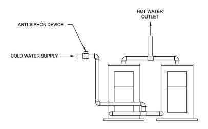
Figure 3 (Dual Water Heater Installation)
