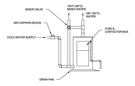
Figure 1 (Dual Temperature System With Mixing Valve)
