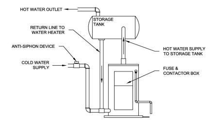
Figure 2 (Single Installation With Storage Tank Gravity Circulation)
