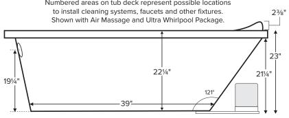
IMPORTANT: Air baths and tubs with a pre-leveled foam base or frame system add 2-3" to overall tub height.
