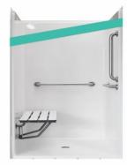
Warm Rain Model FW-4848-B-MN roll-in shower fixtures are constructed of reinforced polyester resin covered with a high gloss gel-coat of 18-20 mils. thickness. The reinforced fiberglass a minimum content of 18% fiberglass.
